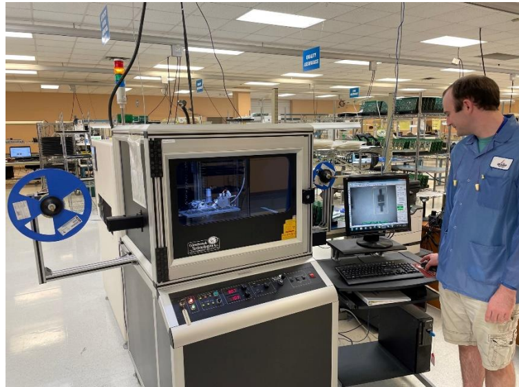
Delta Group Electronics, Inc. uses Glenbrook Technologies’ Jewel Box 70T real-time X-ray system for both quality assurance and counterfeit detection. With the addition of a reel-to-reel accessory, DGEI can verify the authenticity of incoming tape and reel components quickly and easily.
